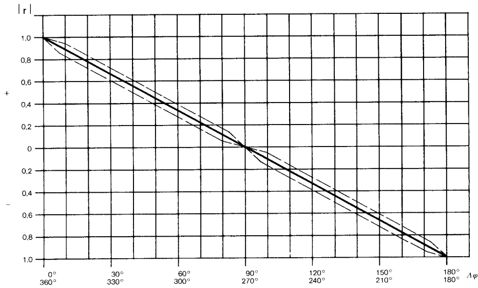
Correlation coefficient r as a function of the phase angle difference \Delta\varphi
